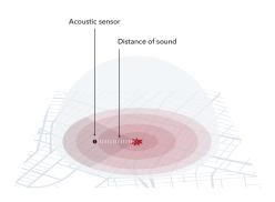
Acoustic sensors throughout the city listen for the distinctive waveforms that firearms produce. When detected, individual sensors calculate the distance to the sound.
