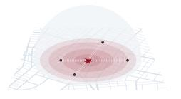
Readings from multiple sensors are used to triangulate the location of the shot.
